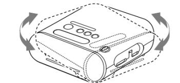
Do not operate the unit over a steel desk or metal surface, as this may lead to interference of reception.
