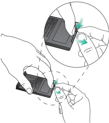
3. Remove the old battery and install the new one with the plus (+) symbol facing up.
