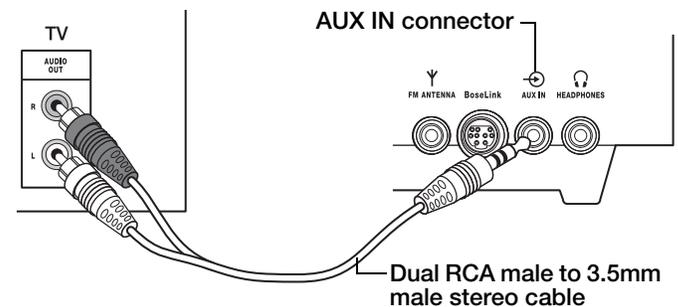
2. Connect the other end of the cable to the **AUX IN** connector on the rear panel of your Wave® music system III.
